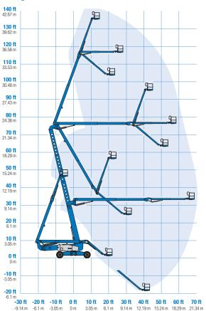
\* The metric equivalent of working height adds 2 m to platform height. U.S. adds 6 ft to platform height. \*\* Gradeability applies to driving on slopes. See operator's manual for
